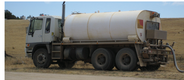
Medium Bulk Water Tanker (10,000 – 16,000L) above with a Heavy BWT above right (16,000 – 35,000L). BWT may be a purpose built tanker or may be a tank(s) mounted on the back of a tip truck, table top truck or on semi trailer. Important for contract tankers to have Storz adaptors for coupling to fire tankers.
