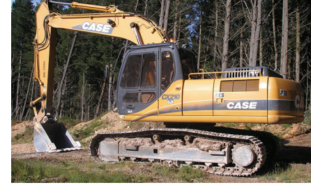
Excavators may be tracked or wheeled. Range in size from Mini (1t) to Large (85t). Able to be configured to perform a broad range of tasks.
