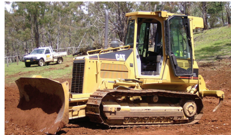
Small (tracked) bulldozer – e.g. Caterpillar model D3 to D5 or Case model 550 to 850. Blade width 2.5 to 3.2m. Mass 8 to 10t.
