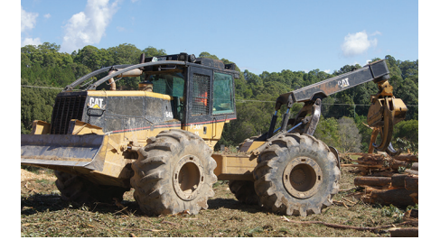
Log Skidders can be tracked or wheeled. Typically used for lifting logs and pushing objects rather than trail construction. Mass 16 to 18t.
