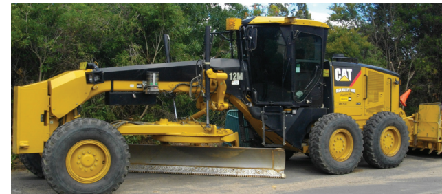
Typically medium in size with blades width 2.4 to 4.3m fitted with ripping tines. May also be fitted with a front blade. Mass up to 25t. Control line construction rates can be between 2 to 6 km/hr.
