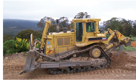
Large tracked bulldozer – e.g. Caterpillar model D8 to D11 or Komatsu model D155 to D575. Blade width 4 to 5m. Mass 31 to 120t.
