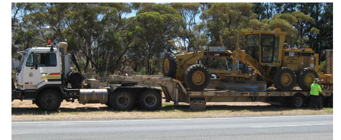
Semi-trailer combination or may be tipper and trailer combination. Assessment of route and staging area to be considered prior to deploying.
