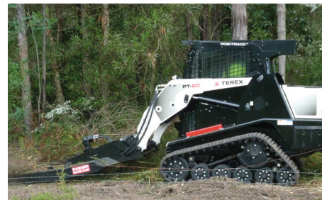
Skid Steer (Bobcat) and Compact Tracked Loader. Bucket capacity 0.5 to 0.7 m 3 . Mass 0.7 to 1.0t.
