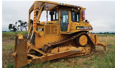
Medium (tracked) bulldozer – e.g. Caterpillar model D6 and D7, Case model 1150 to 1850. Blade width 3.0 to 3.3m. Mass 11 to 30t.
