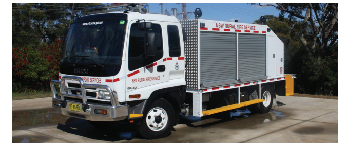
Above is a NSW purpose built field service vehicle, designed to be deployed during campaign fires to provide field (on site) servicing of fire tankers at base camps and assembly areas.
