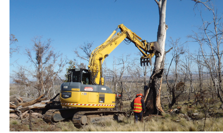
Forest Harvesters may be tracked or wheeled. Designed for harvesting plantation timber even in steep terrain and used for road construction. Mass 25 to 40t.
