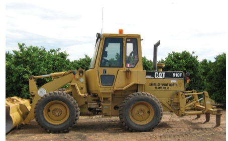
Medium (Wheeled) Loader – e.g. Cat 900 series. Bucket capacity 2.3 to 4.3 m 3 . Mass 15 to 32t.
