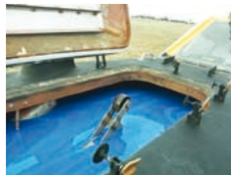
ABOVE LEFT: The buoywall, or portable dam, filled with Phoscheck Aquagel-K before being loaded onto the aircraft. The gel comes in a prilled powdered form, is agitated with water and then pumped into the aircraft for use.
