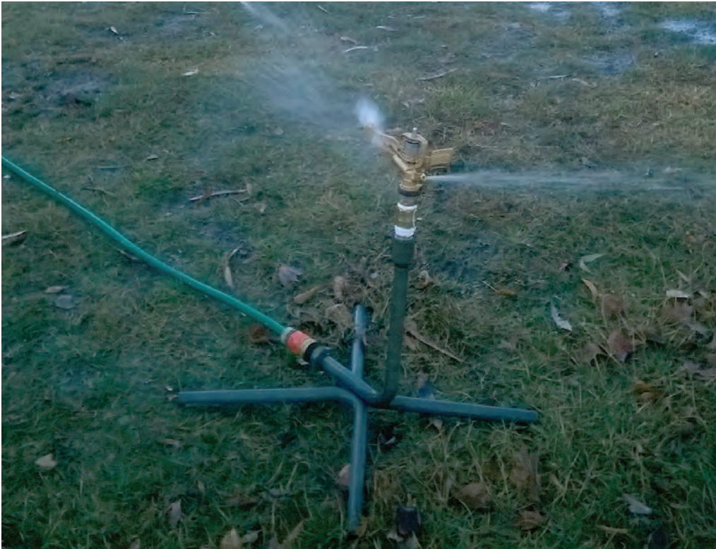
ABOVE: The first step was selecting a suitable sprinkler head and distribution pattern with the available water pressure.
