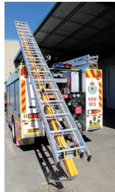
Rescue ladder with gantry lowered
