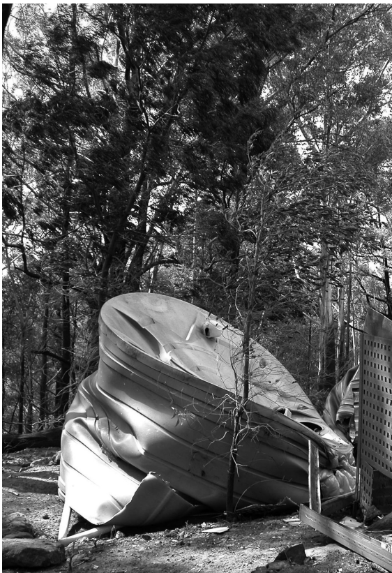
Do not use plastic water storage tanks in bush fire prone areas.
