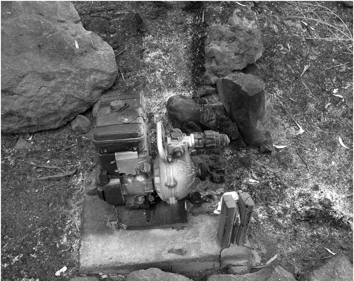
Pumps and other fittings need to be shielded and made of non-combustible materials.
