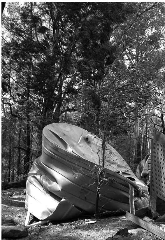
Do not use plastic water storage tanks in bush fire prone areas.
