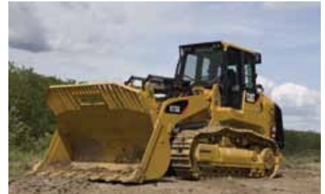
Medium (tracked) Loader – e.g. Caterpillar model 953. Bucket capacity 1.6m 3 . Mass 16t.
