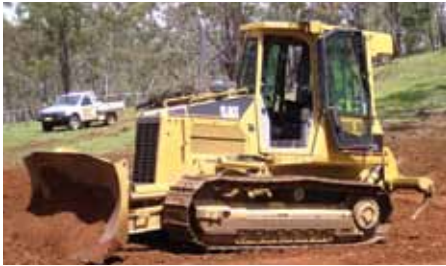
Small (tracked) bulldozer – e.g. Caterpillar model D3 to D5 or Case model 550 to 850. Blade width 2.5 to 3.2m. Mass 8 to 10t.
