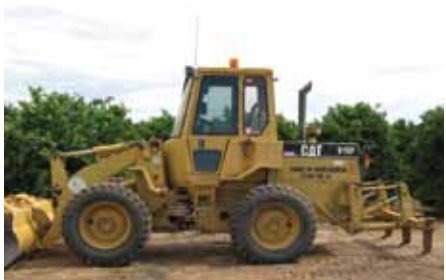
Medium (Wheeled) Loader – e.g. Cat 900 series. Bucket capacity 2.3 to 4.3 m 3 . Mass 15 to 32t.
