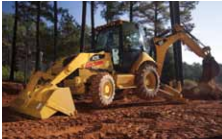
Backhoe Loader series. Bucket capacity 1.0 to 1.53 m 3 . Mass 10 to 12t.
