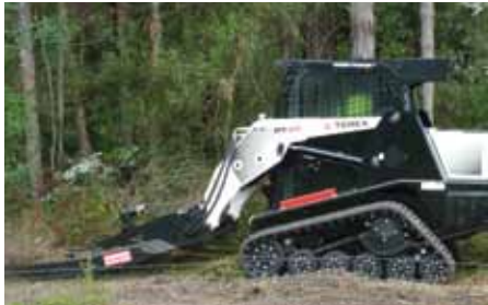
Skid Steer (Bobcat) and Compact Tracked Loader. Bucket capacity 0.5 to 0.7 m 3 . Mass 0.7 to 1.0t.
