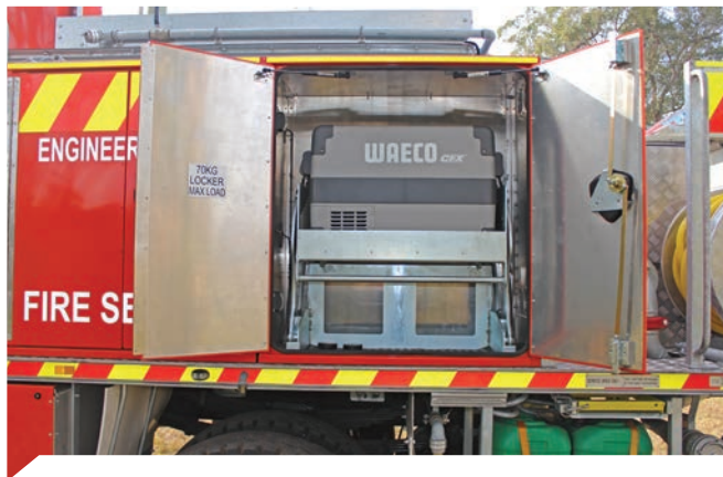
An additional side equipment locker has been added incorporating a drop down holder for portable fridge.
