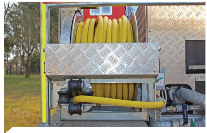
The electric hose reel has been designed with an auto hose lay.
