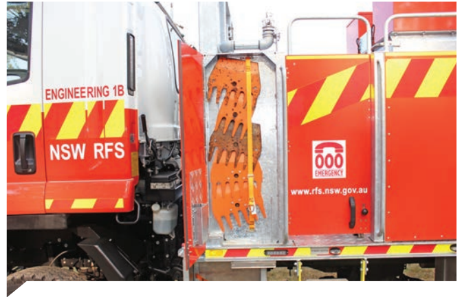
A new headboard incorporates dedicated stowage for five McLeod tools, brush hook, broom, two hydrant bars, storz spanners, 75mm and 38mm suction hoses, floats and strainers. There has also been a re-design of the standpipe stowage.
