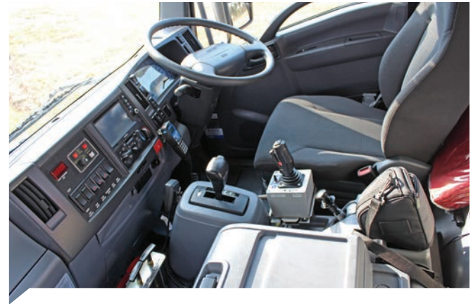
The front monitor is controlled by the operator in the cab through the remote mount controller.
