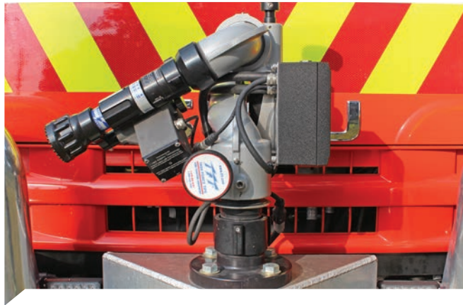
A remote control monitor is mounted on the front bull bar of the new Grasslands Cat 1.
