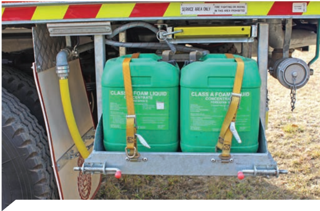
The foam pails are now located in a slide out tray, making it easier to change the pails. The slide out foam storage incorporates stainless steel induction tubes and an induction manifold.
