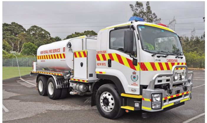
The current build Cat 13 Bulk Water Tanker have an all-white support vehicle paint scheme differentiating them from operational vehicles. Although similar in structure to the new Category 6 tanker, it is without the bull-bar mounted water monitor and shielded crew work area, along with some other minor differences. Photo by Peter Sergeant
