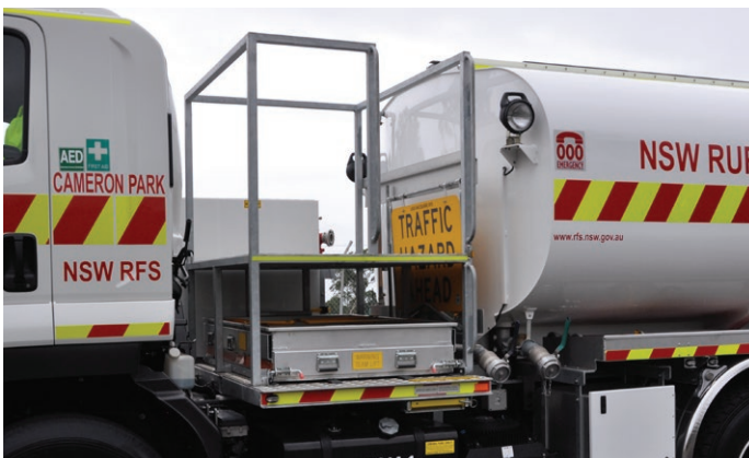
The new Bulky has ample room for a portable buoy wall dam and other equipment behind the cab. Photo by Peter Sergeant
