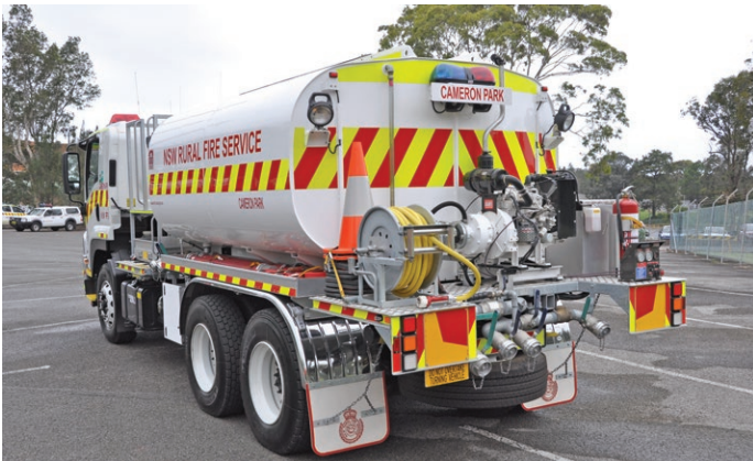
Among the features of the new Cat 13 Bulk Water Tanker is a hose reel that provides flexibility and functionality on the fireground. Photo by Peter Sergeant
