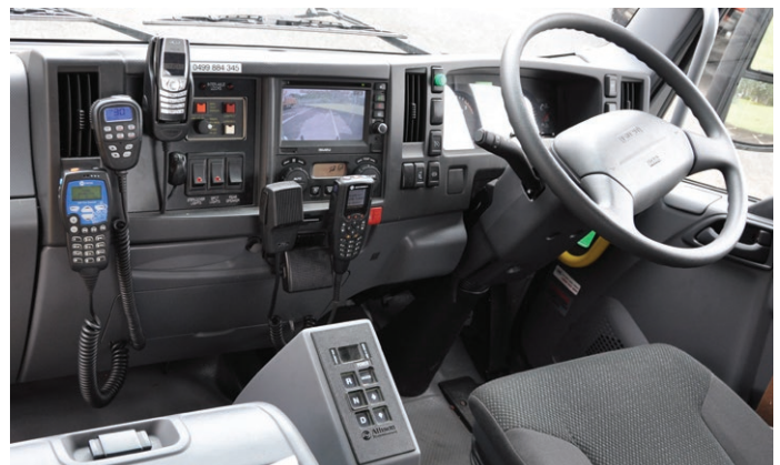
The driver's cab has the usual appointments, however note the push button gear selector. The in-dash multi-function display automatically selects the reversing camera view when reverse gear is engaged. Note the hand-operated transmission retarding lever adjacent to the park brake. Photo by Peter Sergeant
